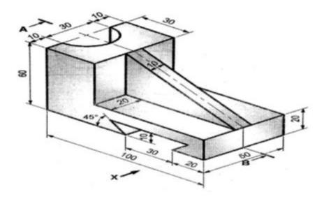
10. From the given figure, Draw (a) F.V, (b) L.H.S.V and (c) T.V using 1<sup>st</sup> angle projection method. Draw the symbol of 1<sup>st</sup> angle projection and show dimensions using aligned method.
