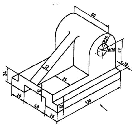
3. From the given figure, Draw (a) F.V and (b) T.V using 3<sup>rd</sup> angle projection method. Draw the symbol of 3<sup>rd</sup> angle projection and show dimensions using unidirectional method.
