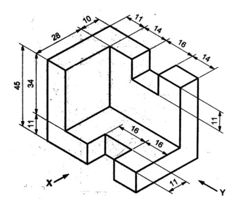
12. From the given figure, Draw (a)F.V and (b)L.H.S.V using  $1^{st}$  angle projection method. Draw the symbol of  $1^{st}$  angle projection and show dimensions using unidirectional method.
