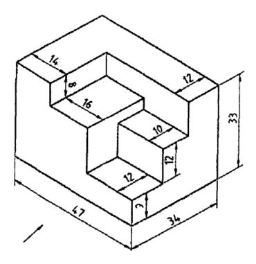
**6.** From the given figure, Draw (a) T.V and (b) F.V using  $1^{st}$  angle projection method. Draw the symbol of  $1^{st}$  angle projection and show dimensions using aligned method.
