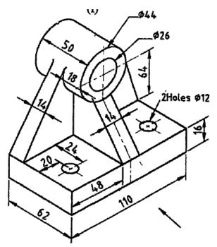
4. From the given figure, Draw (a) F.V and (b) L.H.S.V using 1<sup>st</sup> angle projection method. Draw the symbol of 1<sup>st</sup> angle projection and show dimensions using aligned method.
