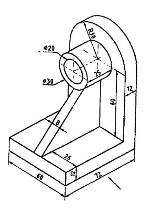
5. From the given figure, Draw (a) F.V and (b) R.H.S.V using 3<sup>rd</sup> angle projection method. Draw the symbol of 3<sup>rd</sup> angle projection and show dimensions using unidirectional method.
