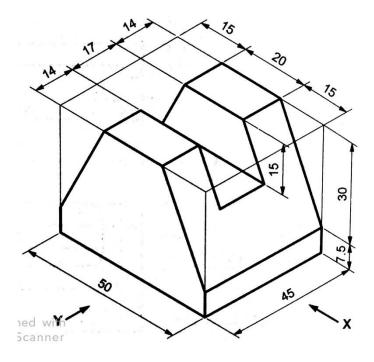
8. From the given figure, Draw (a) F.V and (b) L.H.S.V using 1<sup>st</sup> angle projection method. Draw the symbol of 1<sup>st</sup> angle projection and show dimensions using unidirectional method.
